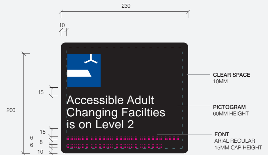
TYPICAL GRAPHIC SETOUT 06: ACCESSIBLE ACCESS - CHANGING FACILITIES (Scale 1:4)
