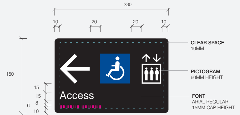
TYPICAL GRAPHIC SETOUT 02: ACCESSIBLE ACCESS (Scale 1:4)
