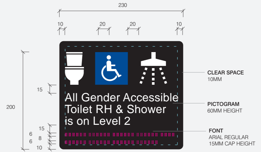
TYPICAL GRAPHIC SETOUT 04: ACCESSIBLE ACCESS - AMENITIES (Scale 1:4)
