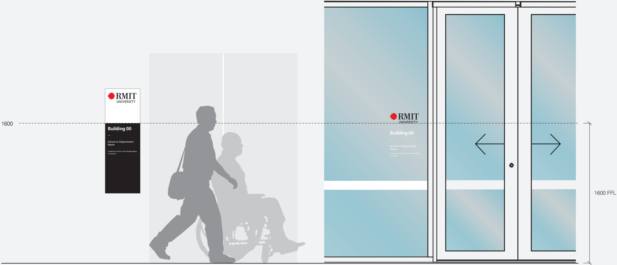
⊖ S.09 BUILDING ENTRY - WALL MOUNTED (Scale 1:25)
