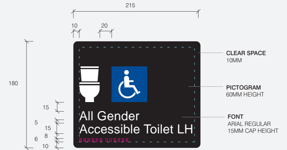
TYPICAL GRAPHIC SETOUT 02: ACCESSIBLE TOILET (Scale 1:4)
